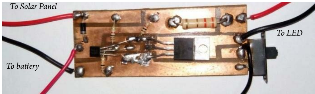
Figure 3b: PCB layout and parts placement by R.Q. Macolor, Solar Night Light , 2013
