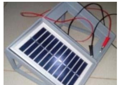
Figure 2c: Solar Panel (Front)
